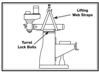
Figure 5. Lifting the mill using web straps.
